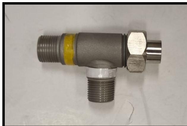
Fig. 3.2: T-fitting with check valve belonging to Taurus Flex 5-1
